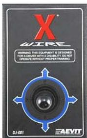
EMC will engineer and install, AEVIT "X-Wire", drive-by-wire systems in the Quovis. This Aerospace Technology (fly-by-wire concepts) has been employed in airplane avionic systems successfully for many years. In "by-wire" systems, the direct mechanical control of a machine is replaced by electronic control. For example, the movement made by the driver with the *joystick*
